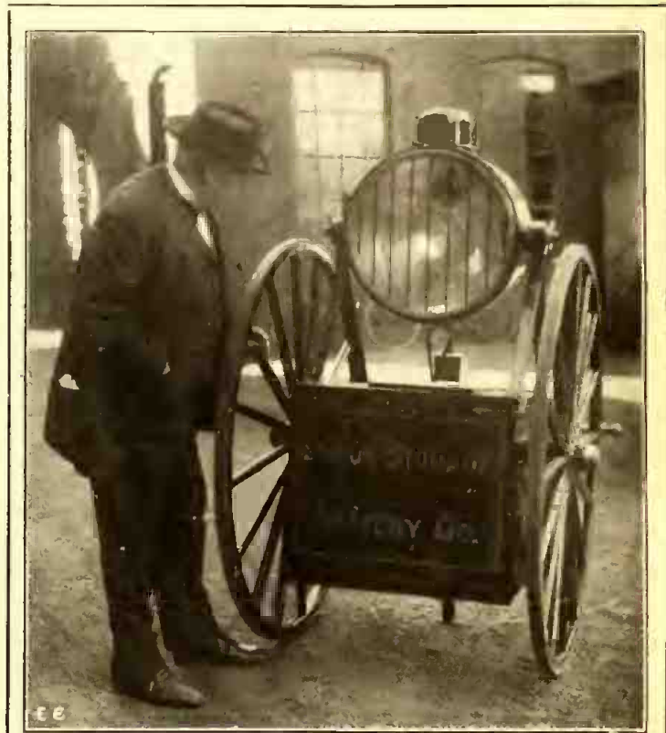
(C) By International News Service. Thomas A. Edison Inspecting His New 3,000,000 C. P. Storage Battery Search Light.
